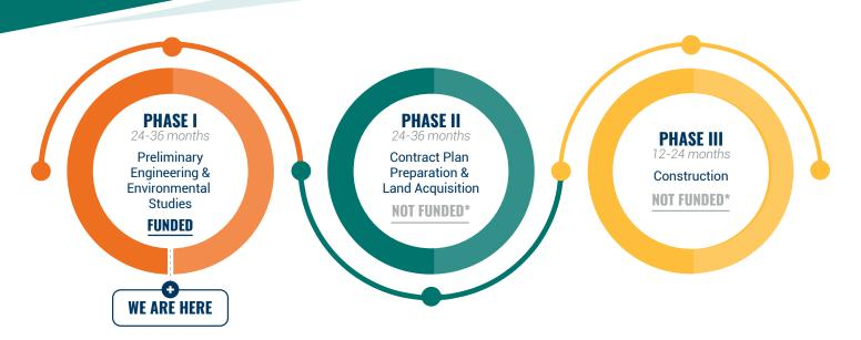
The IL 173 at Keystone Road study is currently in Phase I, which consists of data collection, identification of transportation issues and concerns, development of a range of alternatives, identification of the preferred alternative and its refinement, concluding in approval of an environmental and engineering report which summarizes the study. Phase I is expected to conclude in 2026.
